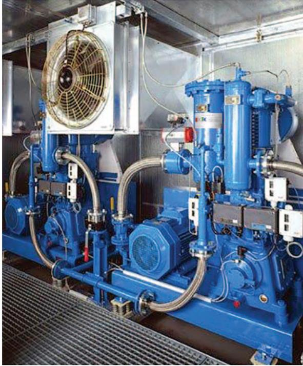
**PDC-PR2-1000-115** two-stage compressor, hydrogen compression for storage, Chemical, 20 barg/289 psig discharge pressure 533 Nm<sup>3</sup>/hr flow rate, 115 kW/154 HP motor.
