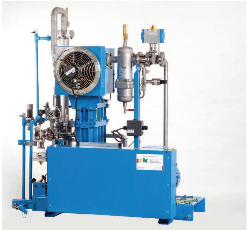
**PDC-P1A-80-15** single-stage compressor, synthesis gas, Petrochemical Industry, 17.9 barg/260 psig discharge pressure, 55 Nm<sup>3</sup>/hr flow rate, 15kW/20 HP motor.
