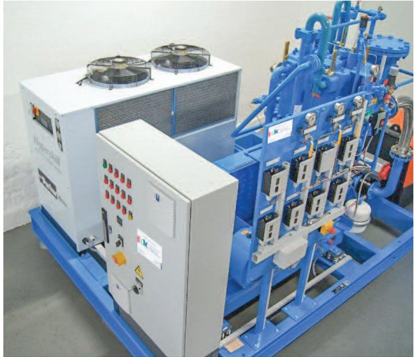
**PDC-PR1-300** single-stage compressor, compression of helium after air separation, Universities & Research Industries, 14 barg/203 psig discharge pressure, 100 Nm<sup>3</sup>/hr flow rate, 22 kW/29 HP motor.
