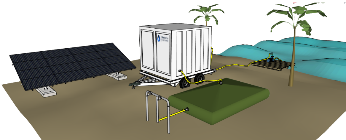
Figure: ROPV System deployed, overall view.
