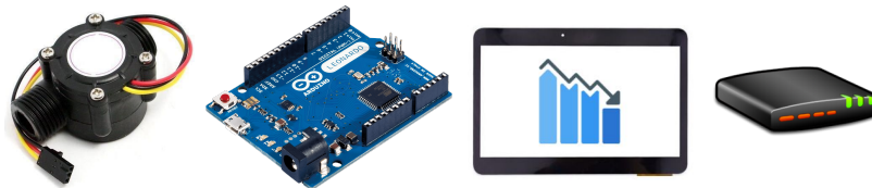
Figure 1. Hardware. From left to right: water flow meter, microcontroller, server computer & screen display
