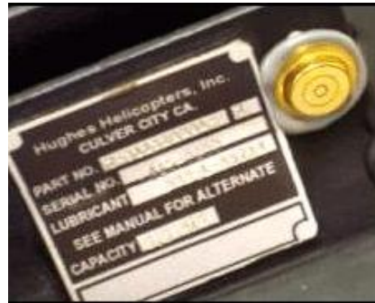
Figure 18.3: CMB attached to a traditional identification plate
