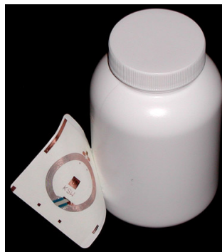
Figure 18.4: RFID tag attached to a medicine
