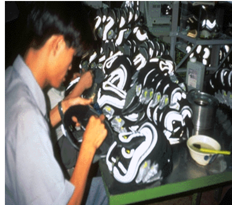
Source: O'Rourke (working on Nike Uppers with glue and solvents and no protective gear") http://web.nmsu.edu/~dboje/TDgreenEYaudit.ht
