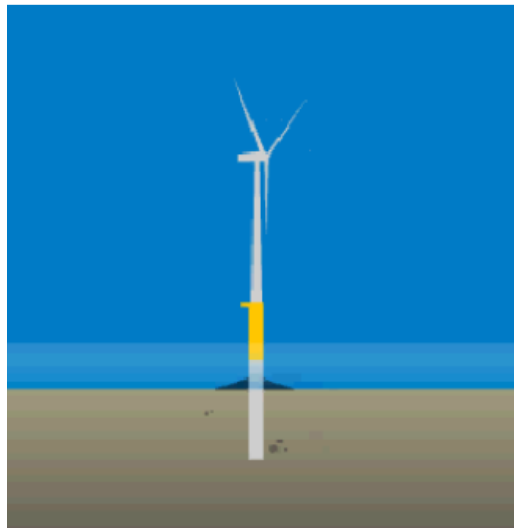
Figure 2.11 Q7 Wind farm monopile model
